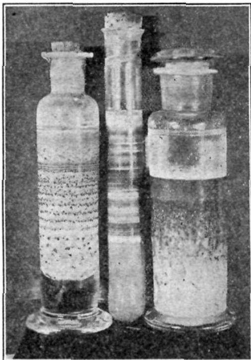
Fig. 2.—Basic mercuric chloride bands. The silicic acid gel on the left contains a slight excess of base, the one on the right a greater excess and the one in the middle contains glucose.
